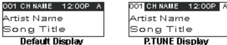
To exit Preset Tune Mode and return to Channel Tuning Mode, press and hold the BAND button.
