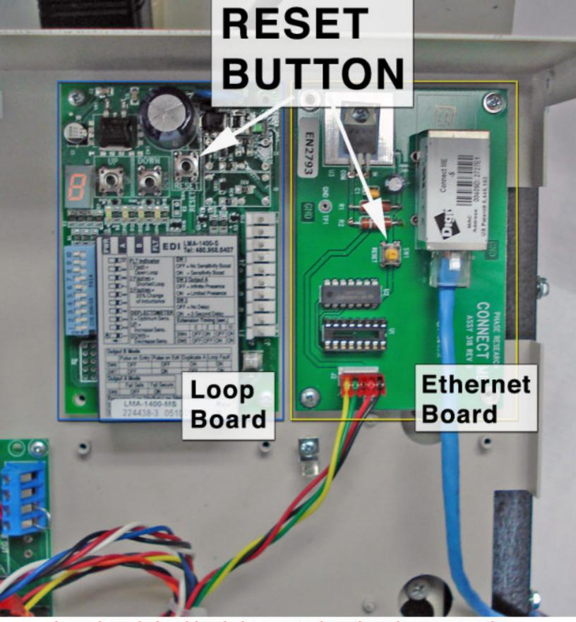
Loop board should only be reset when there is no car at the window. To reset either board, give the button a good push and let go. This picture shows the "Connect Me" ethernet card and the EDI style loop board. If you have a different loop board, please refer to the "Fast Track loop board ID" document. If you have a different ethernet card, refer to the "Fast Track ethernet ID" document.
